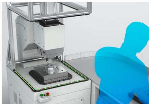
Multi-sided protection using series connection
