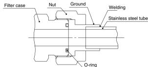
Weld the ground and piping when the fitting is used. At the time of welding, supply inert gas such as Nitrogen to the piping to prevent the formation of an oxide film. Also, remove the oxide film on the external surface through electrolytic polishing or acid cleaning.
