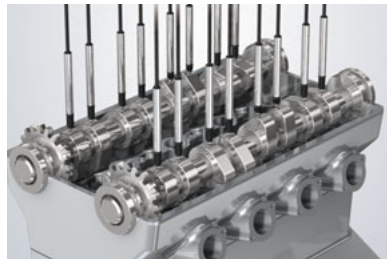
Camshaft runout measurement
