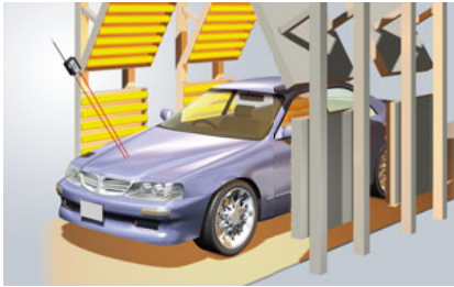
Measuring temperature in painting process
