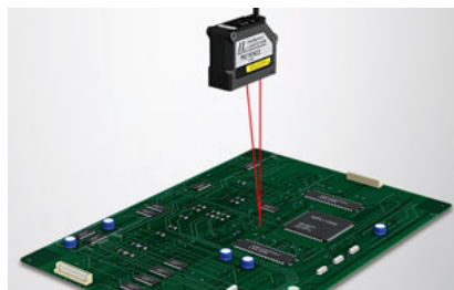
Height controls of a PC board
