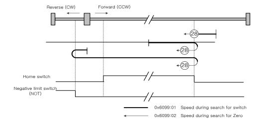
The initial driving direction is reverse (CW), and a point where the Positive Home Switch is turned on becomes the Home position.
