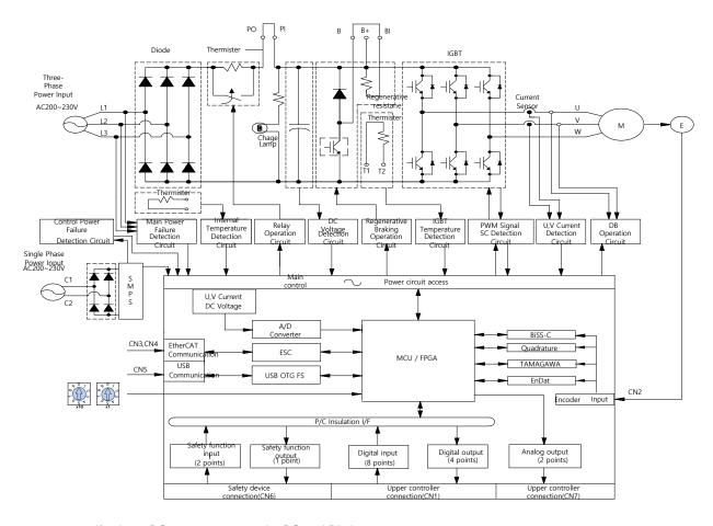
If using a DC reactor, connect the PO and PI pins.
