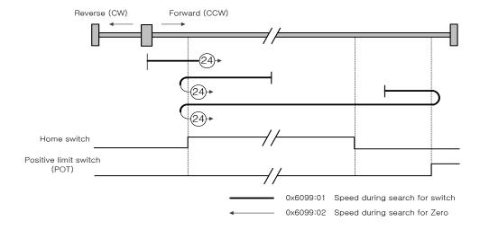
The initial driving direction is forward (CCW), and a point where the Positive Home Switch is turned on becomes the Home position.
