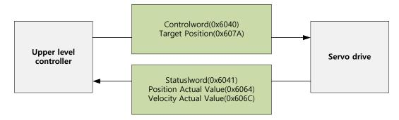
This is an example when assigning the Controlword and the Target Position with the RxPDO (0x1600).
