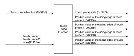
The position value of the encoder (Actual Position Value, 0x6064) is latched by the following trigger events according to the setting value. At the same time, 2 channel inputs can be latched independently at the positive/negative edges.
