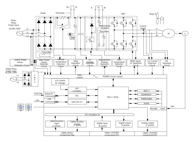
Note 1) If using a DC reactor, connect the PO and PI pins.
