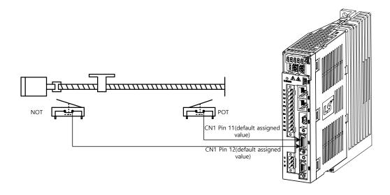
If the Forward/Reverse limit signals are input, the motor will stop according to the emergency stop setting (0x2013).
