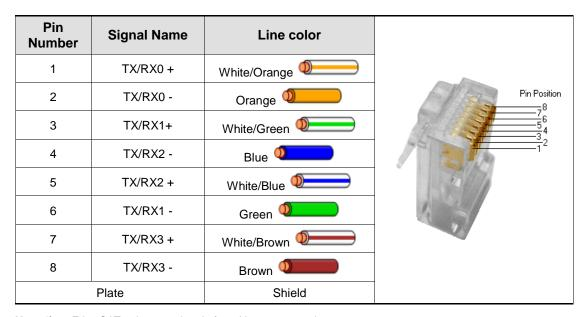
Note 1) EtherCAT only uses signals from No. 1, 2, 3, and 6.
