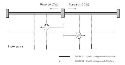
The initial driving direction is reverse (CW) for the method 33, and forward (CCW) for the method 34. The drive detects the index pulse at the Zero Search Speed.
