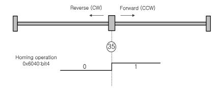
The current position at startup of homing operation becomes the Home position. This method is used to change the current position to the origin depending on demand of the upper level controller.
