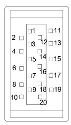
**Analog Monitor Connector specification : DF-11-4DS-2C (HIROSE)**
