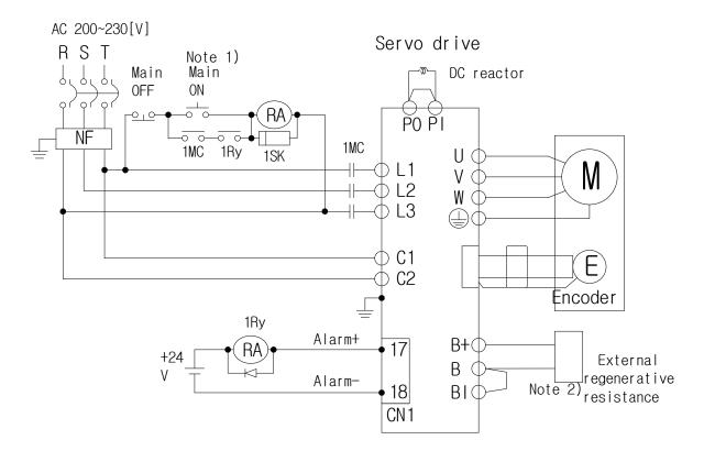
**Note 1)** It takes approximately one or two seconds to output an alarm signal after turning on the main power. Accordingly, press and hold the main power ON switch for at least two seconds.
