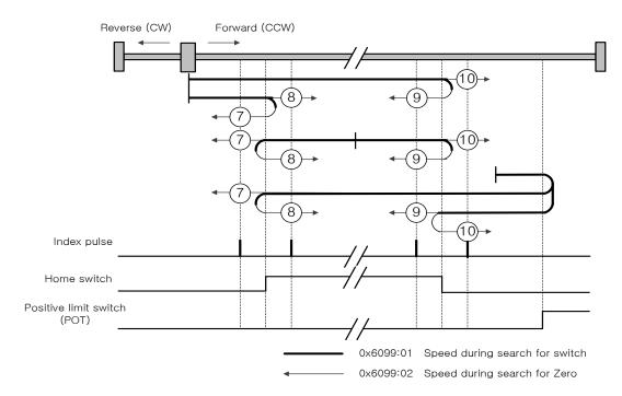
For homing using the Homing Method 7, the velocity profile according to the sequence is as follows. The sequence depends on the relationship between the location of load and the Home switch at homing, which is categorized into three cases as below. For more information, see the details below:
