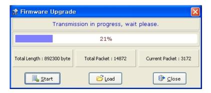
6) After clearing, the firmware is transmitted automatically and the progress bar and "Current Packet" display the current transmission status. (The transmission time depends on the PC performance, but it usually takes from scores of seconds to several minutes.)
