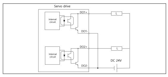
Note 1) For DO1 and DO2 output signals, the GND24 terminal is separated.
