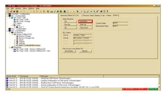
**3.** After the current state is changed to BOOT and you check the drive status (ERR LED ON), wait for approx. 10 seconds until the internal flash memory of the drive is cleared.
