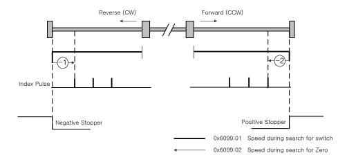
Homing methods -1 and -2 are using Stopper and Index (Z) pulse to home. The velocity profiles depending on the sequence are shown below. For more information, see the details below:
