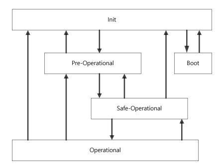
The EtherCAT drive has 5 states as above, and a state transition is done by an upper level controller (master).
