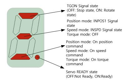
Digit5 indicates state of EtherCAT State Machine, current control mode or state of servo on.
