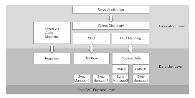
This drive supports a CiA 402 drive profile. The Object Dictionary in the application layer includes application data and PDO (Process Data Object) mapping information from the process data interface and application data.
