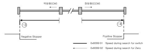
Homing method -3 and -4 are using Stopper to home. The velocity profiles depending on the sequence are shown below. For more information see the details below.
