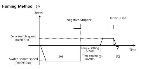
(A) The initial driving direction is reverse (CW), and the drive operates at the Switch Search Speed.
