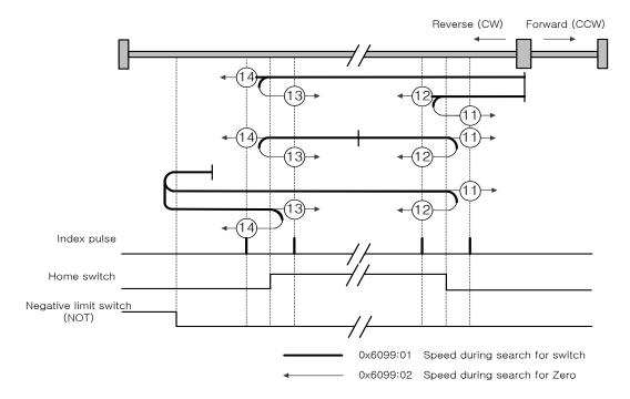
For homing using the Homing Method 14, the velocity profile according to the sequence is as follows. The sequence depends on the relationship between the location of load and the Home switch at homing, which is categorized into three cases as below. For more information, see the details below:
