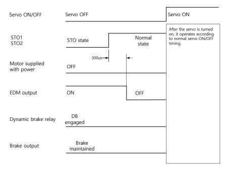
Note 1) Be sure to recover the input signals of STO1 and 2 to ON at the servo OFF state. It is not necessary to reset alarm separately since the "STO state" is not an alarm state.
