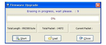
5) Press the "Start" button to start transmission. 10 seconds are counted down to clear the internal memory in the drive. (For XDL-L7NH and L7P, the segment 7 should display "USB". For PEGASUS, a red "ERR" LED should be illuminated.)
