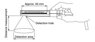
The measurement of a part with a high-charge potential can be highly dangerous as it can cause a discharge to the user's hand.
