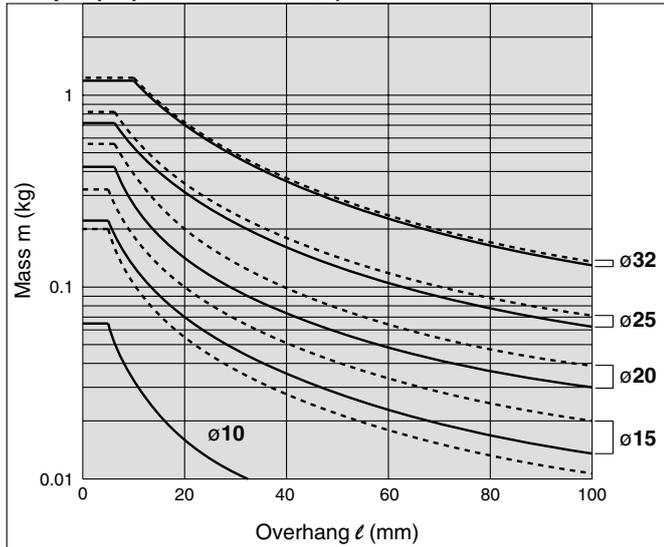
**Graph (15) V = Over 400 mm/s; Up to 100 mm stroke** ——— CXSJM
