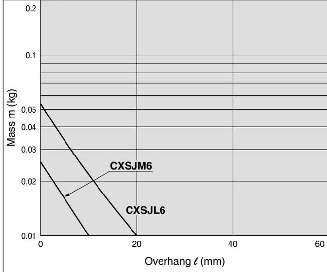
**Graph (10) V = Up to 400 mm/s; Up to 30 mm stroke** ——— CXSJM
