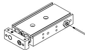
2. To unlock, pull the manual lever in the direction of the arrow. Release the manual lever to return the cylinder to a ready-to-lock state.
