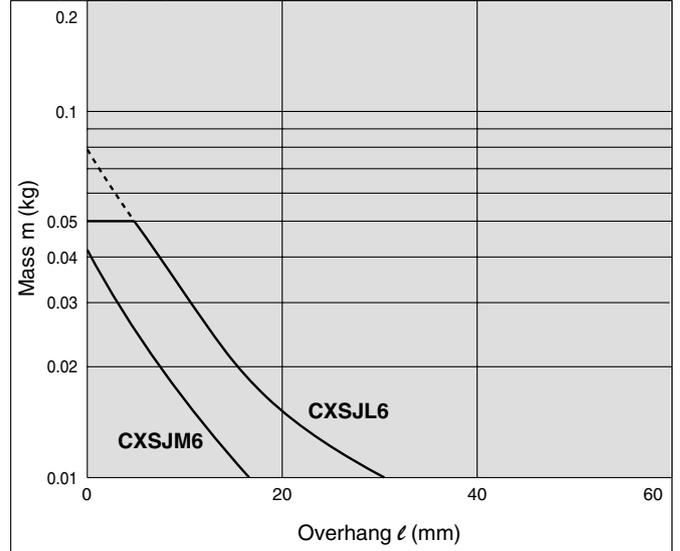
**Graph (8) V = Up to 400 mm/s; Up to 10 mm stroke** ———— CXSJM
