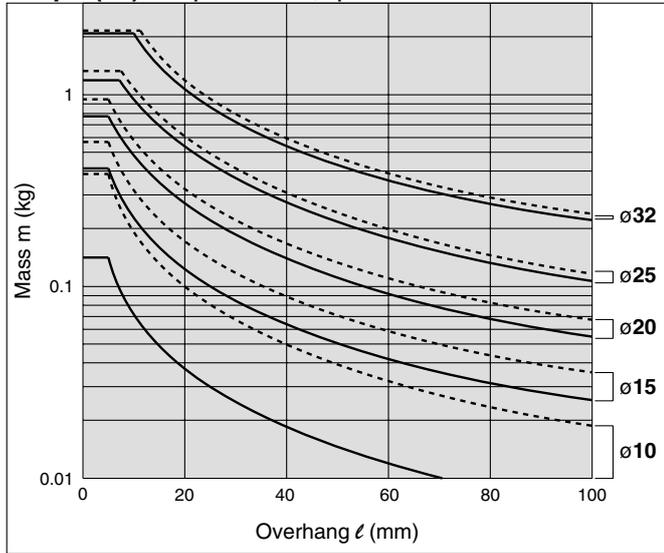
**Graph (11) V = Over 400 mm/s; Up to 30 mm stroke** ——— CXSJM
