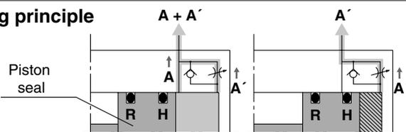
1. When the piston is retracting, air is exhausted through both A and A' until piston seal H passes air passage A.
