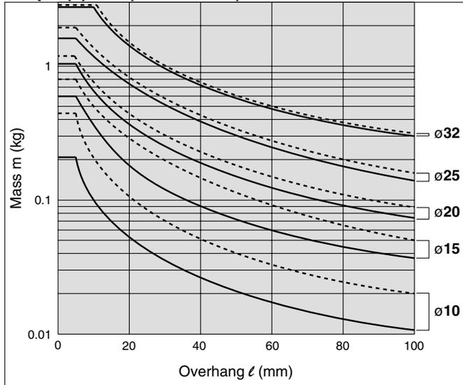
**Graph (9) V = Over 400 mm/s; Up to 10 mm stroke** ———— CXSJM
