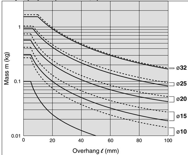
**Graph (13) V = Over 400 mm/s; Up to 50 mm stroke** ———— CXSJM
