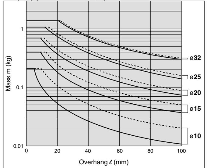
**Graph (12) V = Up to 400 mm/s; Up to 50 mm stroke** ———— CXSJM
