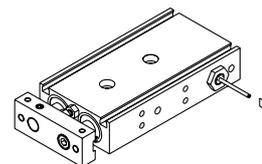
3. The manual lever ( $\phi 1.6 \times 35 \ell$ , tip part: M1.6 x 0.35 x 3  $\ell$ ) is included with the cylinder. If additional manual levers are required, use the following part number to place an order: CXS06-48BK2777 (for all series).
