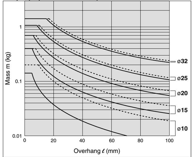
**Graph (14) V = Over 400 mm/s; Up to 75 mm stroke** ——— CXSJM
